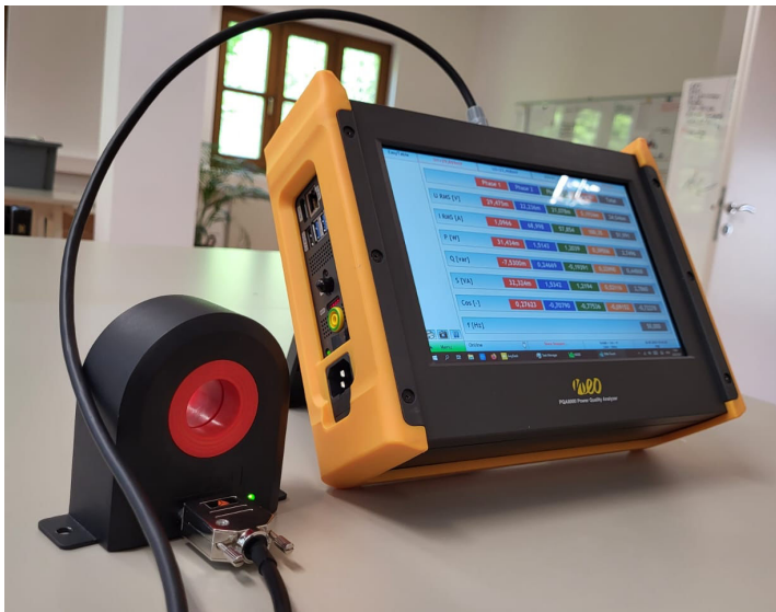
Figure 7: Danisense fluxgate current transducer in combination with the PQA8000 from Neo Messtechnik
