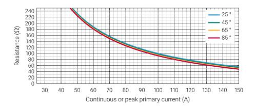
Figure 2: Maximum measurement resistor R<sub>M</sub> vs. current and ambient temperature
