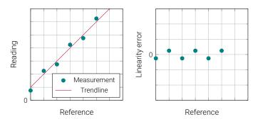
Figure 1: Linearity error definition
