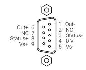
Figure 6: DSUB-9 connection pinout
