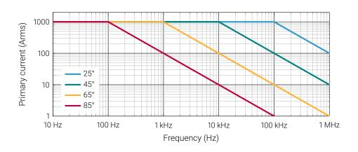
Figure 4: Maximum continuous primary current vs. frequency
