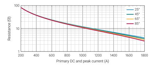
Figure 2: Maximum measurement resistor  $R_{\mbox{\scriptsize M}}$  vs. ambient temperatures
