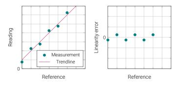
Figure 1: Linearity error definition
