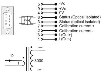
When sensor is operating in normal condition the status pins are shorted.
