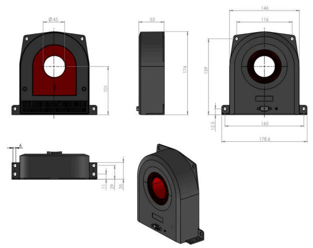
Dimension in mm (general tolerance 0.3mm unless otherwise stated)
