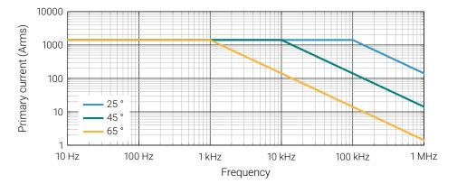
Figure 2: Maximum continuous primary current vs. frequency
