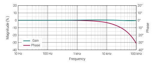
Figure 3: Frequency characteristics
