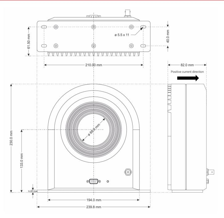
Figure 4: Dimensions of transducer. 0.3 mm Tolerance
