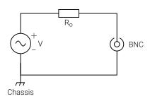
Figure 7: BNC shield and chassis connection
