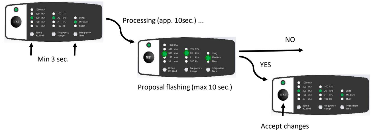
NB: Frequency range of 100Hz is not included in the auto setup feature i.e. if desired the user must select it manually. The RCM will always give priority to settings which make the RCM more sensitive i.e. higher frequency ranges and shorter integration times.
