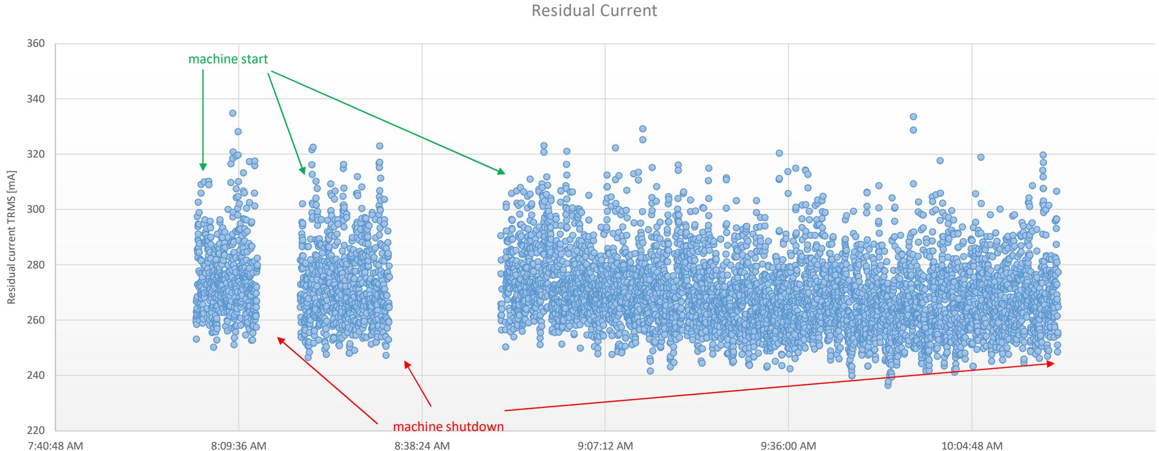
Due to the integration interval over **1000 ms**, the current peaks during switch-on and switch-off processes are smoothed, so that no clearly increased values are recognizable via the TRMS calculation.
