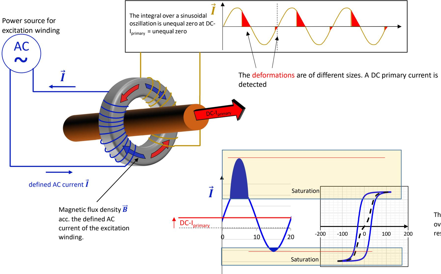
The magnetic flux density  $\vec{B}$ , averaged over a complete sinusoidal oscillation, results in zero.
