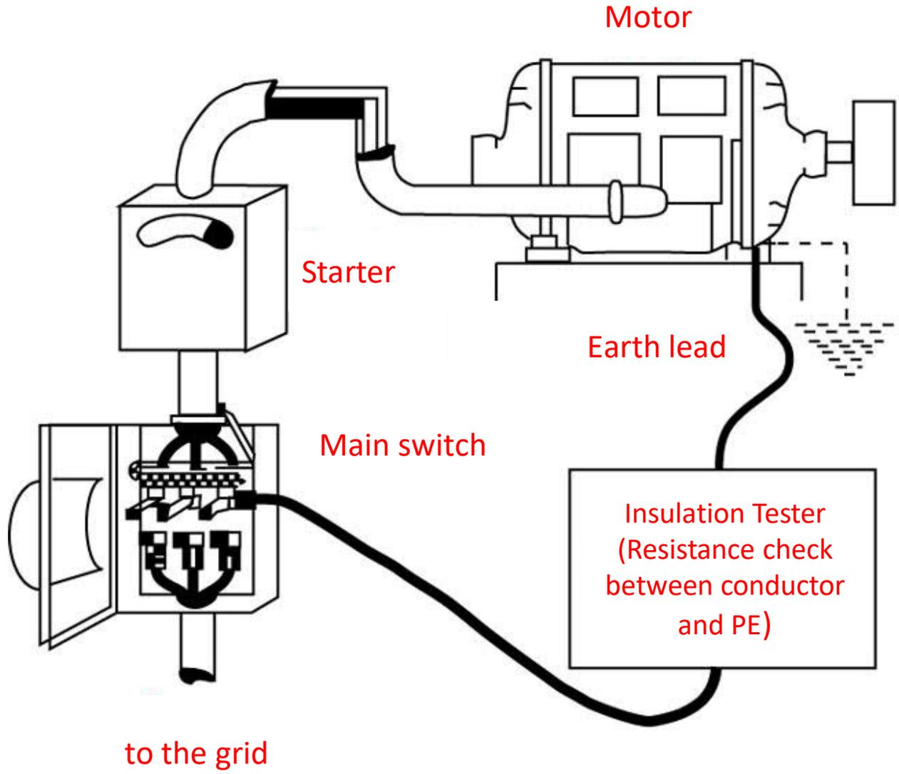
The insulation resistance must be measured between each active conductor and the protective conductor or earth.
