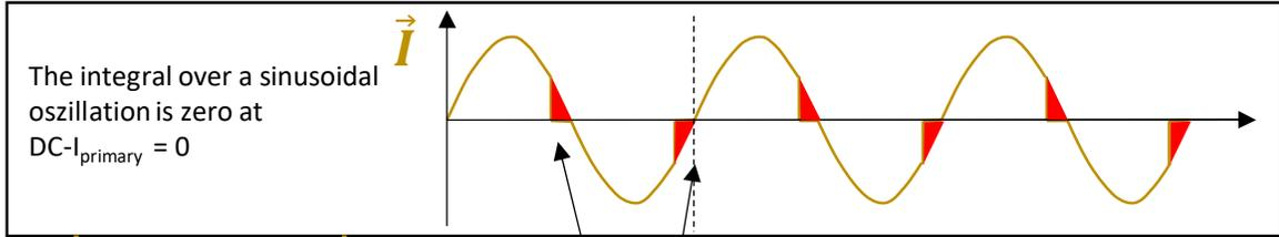
The deformations are the same. No DC primary current is detected
