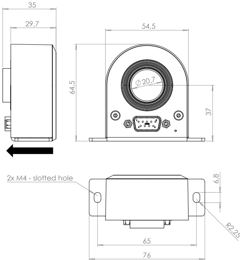
Figure 5: Dimensions of transducer. 0.3 mm Tolerance
