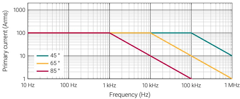
Figure 3: Maximum continuous primary current vs. frequency
