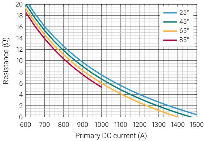
Figure 2: Maximum measurement resistor  $R_M$  vs. ambient temperatures
