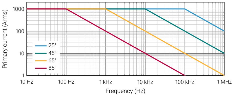
Figure 4: Maximum continuous primary current vs. frequency
