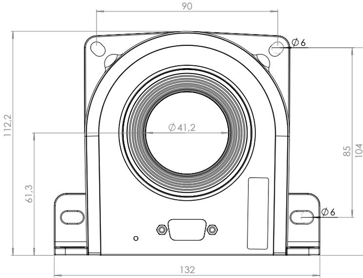
Figure 6: Dimensions of transducer. 0.3 mm Tolerance
