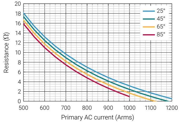
Figure 3: Maximum measurement resistor  $R_M$  vs. ambient temperatures
