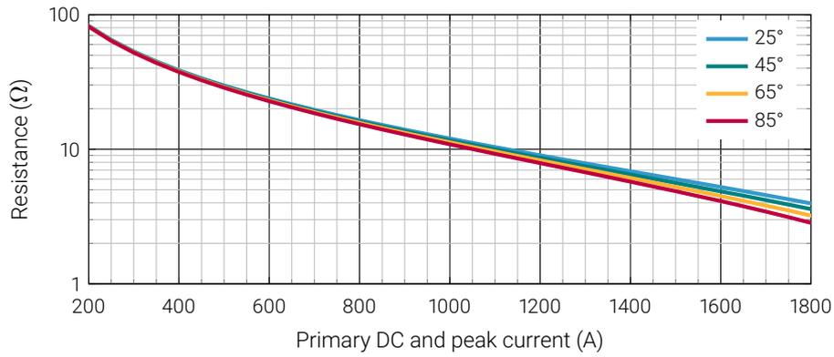
Figure 2: Maximum measurement resistor  $R_M$  vs. ambient temperatures
