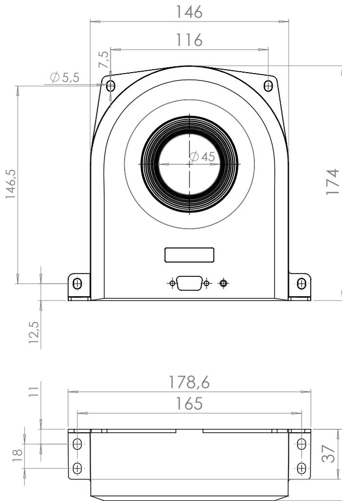
Figure 5: Dimensions of sensor head. Tolerance is 0.3 mm
