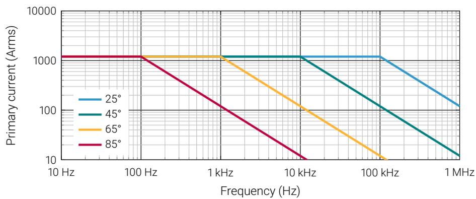
Figure 3: Maximum continuous primary current vs. frequency
