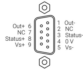
Figure 6: D-sub-9 connection pinout
