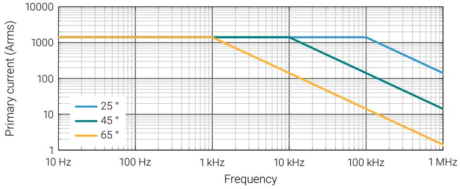
Figure 2: Maximum continuous primary current vs. frequency
